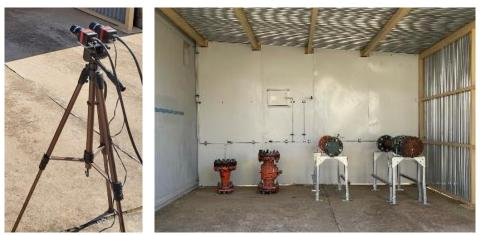
Figure 10. EM during validation campaign at ENAGÁS Zaragoza calibrated test bench
