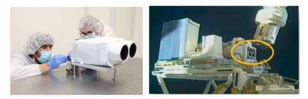
Figure 5. iSIM-90 VNIR camera for CASPR mission. Left: At SATLANTIS clean room. Right: At the ISS in the NASA modules
