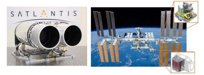
Figure 9. iSIM-170 IOD mission. Left: At SATLANTIS. Right: At the ISS (bottom right)
