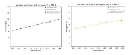
Figure 11. EM validation with the gas cell. SpectraPlot © values (dots) vs EM measurements (crosses) and fit (dashed lines)
