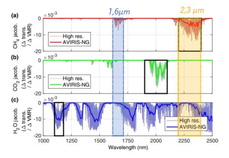
Figure 8. CH4 absorption at 1600 and 2300 nm [2]
