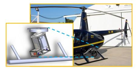
Figure 14. PM setup in a helicopter
