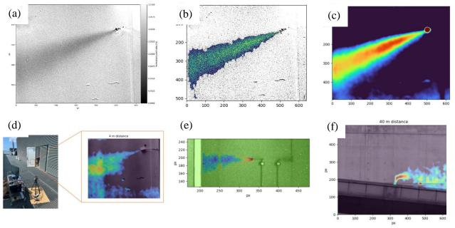
Figure 12. EM field tests and color maps indicating different CH4 concentrations at different distances: 4 m (a, b, c, d), 17 m (e) and 40 m (f)
