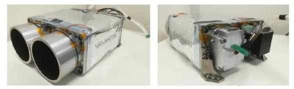
Figure 3. PM (Plane Model) fully integrated design of the opto-mechanics of iSIM-90 SWIR. The FM (Flight Model) will be slightly different, as a different VNIR detector will be used.
