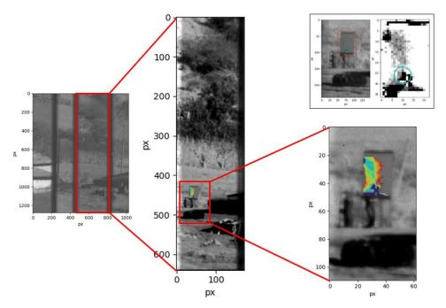
Figure 13. PM field test and color map indicating different CH4 concentrations at 1 km distance
