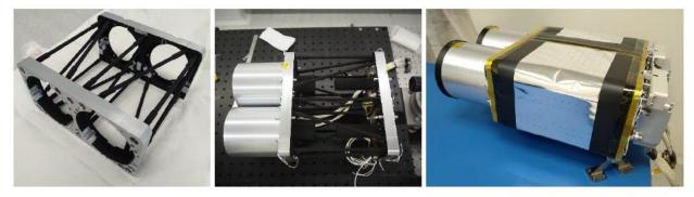
Figure 4. iSIM-90 VNIR camera for CASPR mission during integration at SATLANTIS
