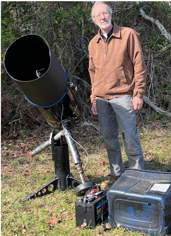
Fig. 7. Roger Venable with one of his 36cm SCTs with Fastar modification and a large dew shield. The large battery is used to power his recording and timing equipment, not the telescope, which is manually pointed to the altitude and azimuth of the occultation using stars.
