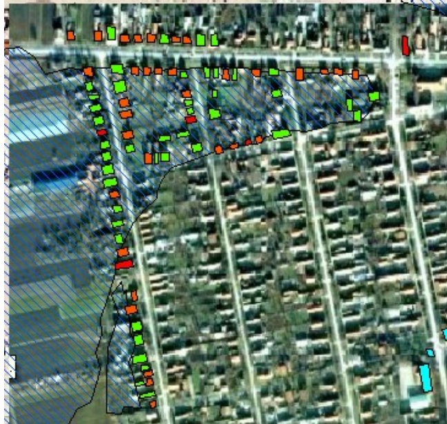
Figure 4. Structural vulnerability of individual houses with an assigned color (degree of structural vulnerability) overlapped with simulated flooded area based on DEM and historical disaster database. [6]
