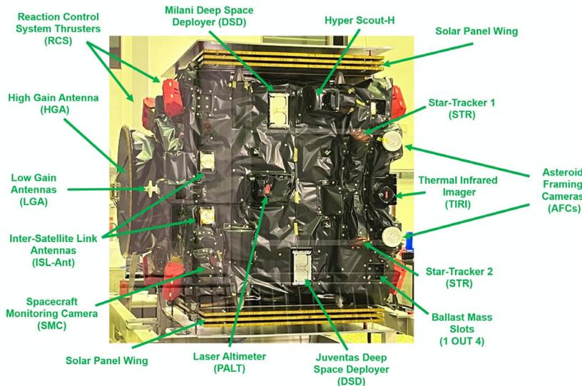
Figure 4a. Hera S/C Instruments description, on Asteroid deck (Image Credit OHB Systems/ESA-2024)
