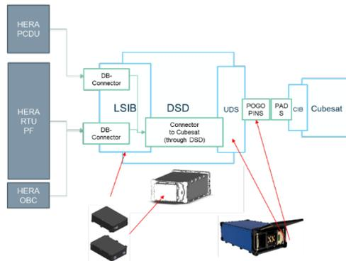
Figure 11d –LSIB+DSD+Hera high level schematics.
