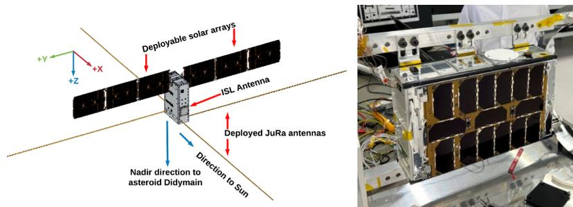
Figure 8 – Deployed (Render, Left) and Stowed (Flight Unit, right) configuration of the Juventas satellite
