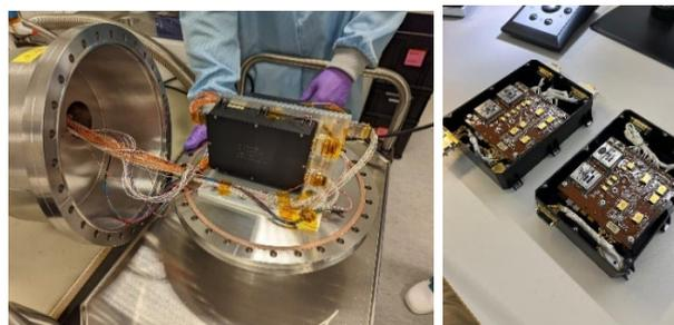
Figure 11c – Juventus and Milani Life Support Interface Board (LSIB) FMs serving as interface with the Hera Satellite.
