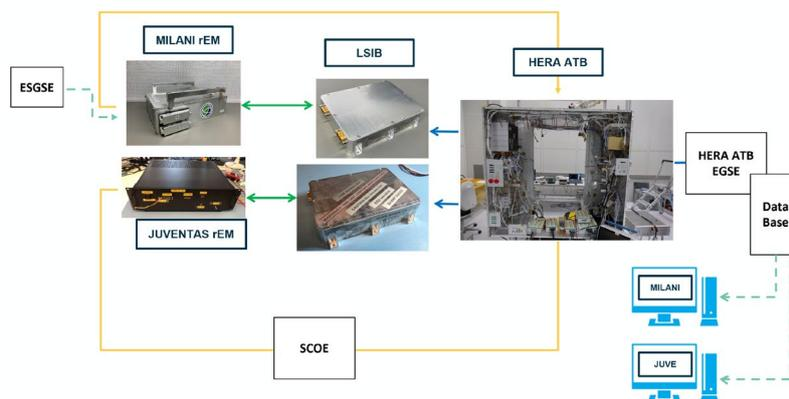
Figure 14 – Milani and Juventas rEMs connected to the Hera ATB at OHB Bremen Clean Room (Image Credit OHB Systems/ESA)
