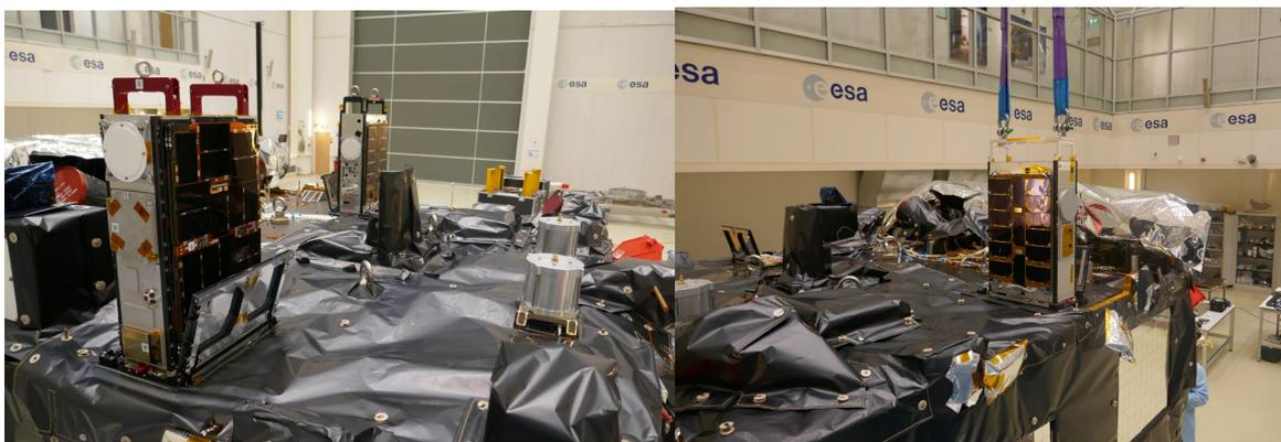
Figure 21. Hera Cubesats PFMs in Exposed Configuration during the Exposed Checkouts functional tests at ESA Rosetta clean room (Image credit OHB Systems and ESA). MGSE + Slings + Clean room crane used as off-loading system during the Hot deployment of the CRS
