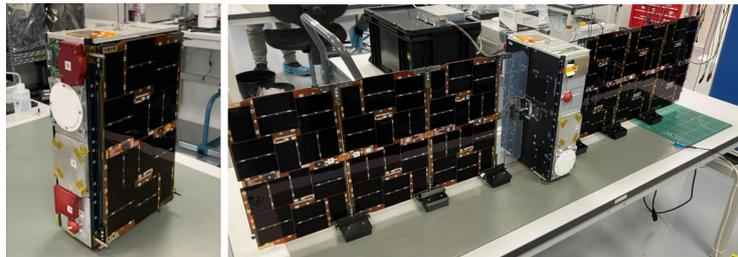
Figure 5. 6U-XL Milani CubeSat (Flight Units) stowed and deployed configurations (image credit: Tyvak International)
