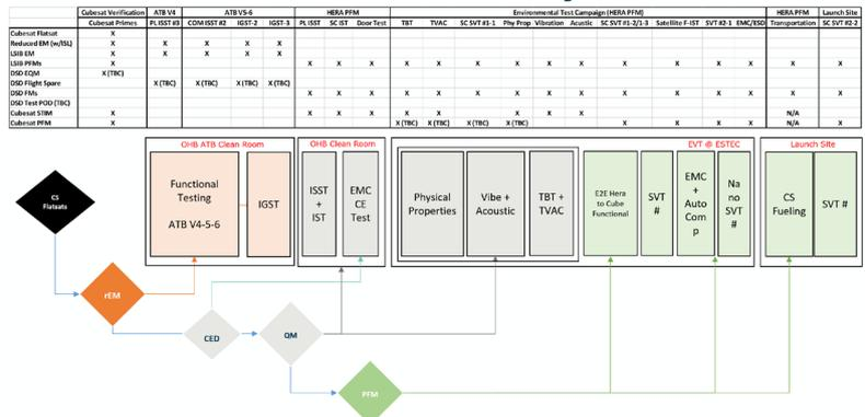
Figure 13. Hera AIT Flow Vs Hera CubeSat Models. Reduced Engineering Model (rEM), Conducted Emission Model (CED), Qualification Mode (QM), Proto-Flight Models (PFM)
