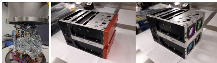
Figure 1. ASPECT Payload Flight Unit (Image credit of VTT)
