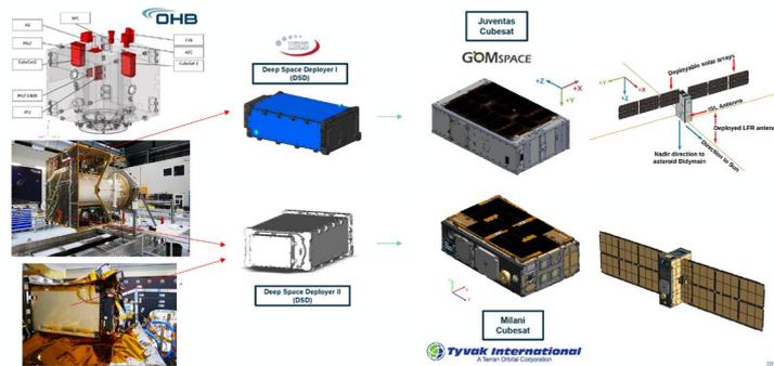
Figure 4b. Deep Space Deployers and CubeSat accommodation on Hera
