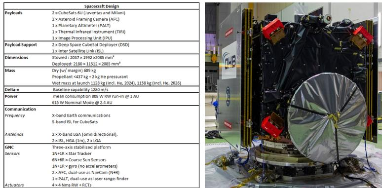
Figure 4 – Hera S/C characteristics (left) and Hera platform during vibration testing (right) (Image Credit OHB Systems)
