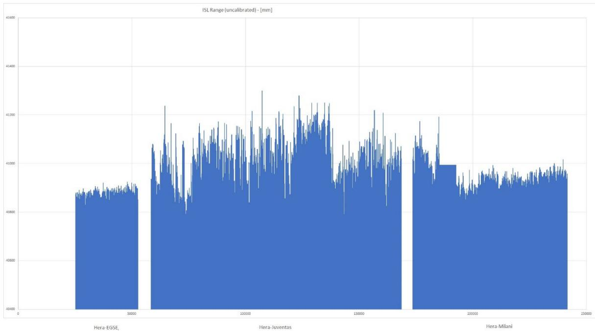
Figure 21a. Ranging Measurement obtained from Hera ISL while connected to Hera Cubesats on TestCaps, without any post-processing or calibration.
