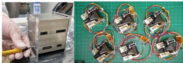
Figure 9 – Juventas Low-Frequency Radar Flight Unit(left) (Image credit: IPAG and Emtronix Lux.). Low-Frequency Radar Antennas Flight Models (Right). (Image credit: Astronika)
