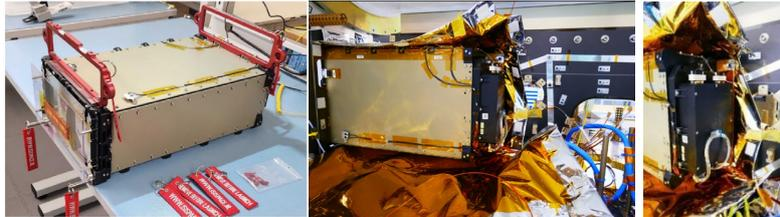
Figure 11b – Deep Space Deployer (Stand-alone, Image Left credit ISISpace NL). Deep Space Deployer + LSIB integrated inside Hera S/C (image in the right, credit OHB Systems)
