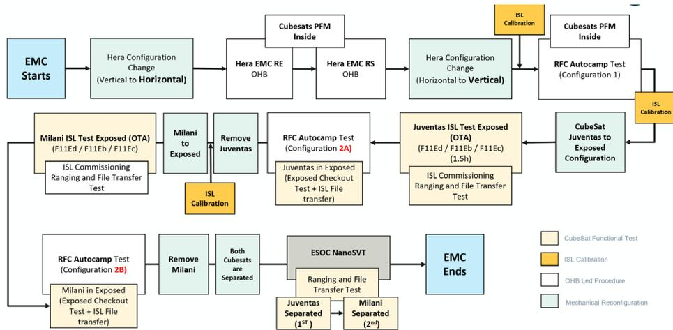
Figure 22. EMC and Auto-compatibility testing flow for Hera and the Hera Cubesats. Tests executed at the ESA Maxwell Anechoic chamber facility.
