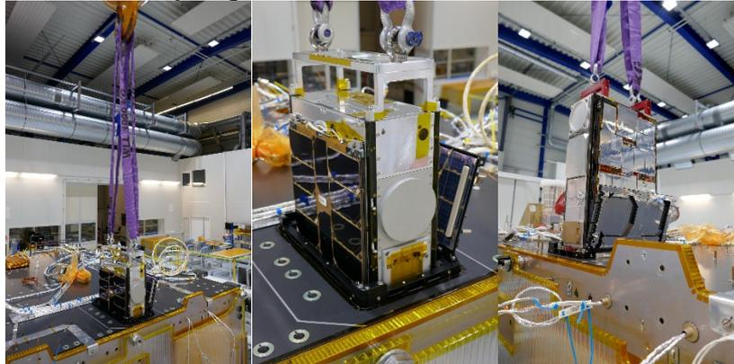
Figure 16 – Milani (right image) and Juventas (2xleft) Qualification Models being integrated on the Hera platform, showing its integration MGSE and utilising the clean room crane (Image credit OHB Systems/ESA)
