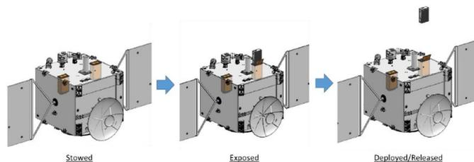
Figure 12: Illustration (Credit OHB Systems) of the two-step CubeSat deployment sequence. Left: The CubeSat is stowed inside the DSD (highlighted in orange). Middle: The CubeSat is ejected from the DSD into the exposed configuration, but still connected to the spacecraft for power and communication. In this configuration, the ISL RF communication link shall be established. Right: The CubeSat is released and separated from the spacecraft
