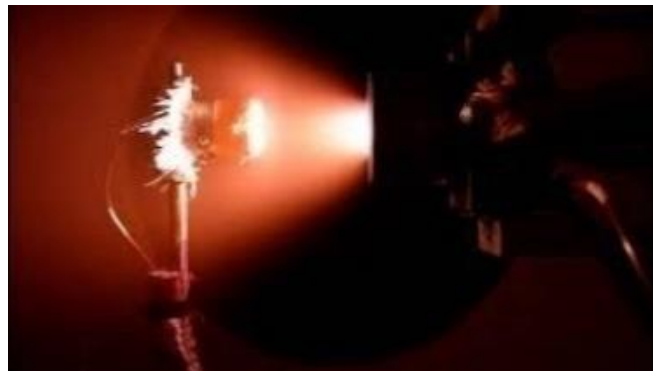
Figure 8: CNRS-ICARE Plasma wind tunnel test
