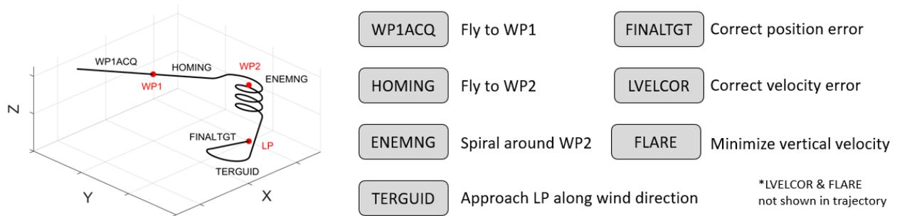
Figure 1. SR RM parafoil guidance phases
