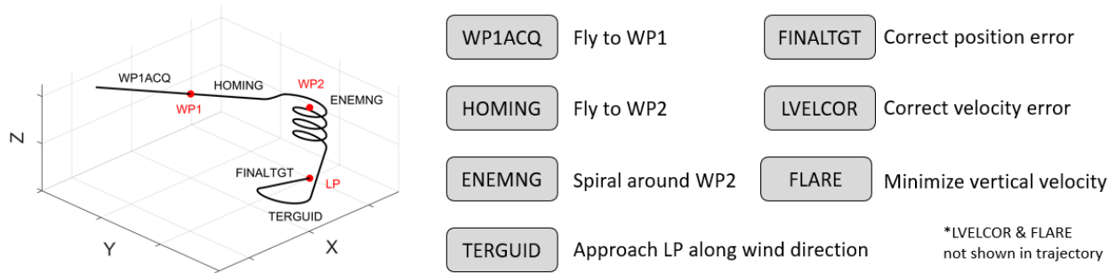
Figure 1. SR RM parafoil guidance phases
