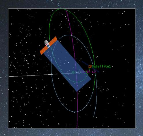
Without performing any manoeuvre, LICIAcube would be travelling for 6-months (the planned extended mission duration) along the inner DRO trajectory branch thus satisfying the planetary defence scenario for detecting imminent impactors.
