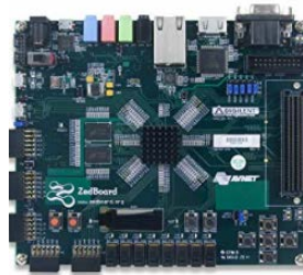
Figure 1: Digilent 410-248 ZedBoard Zynq 7000 Development Board © Xilinx
