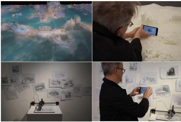
Figure 6: Different facets of the AR experience. (Upper) A projection on a 3D landscape with embedded marker for using AR to show the 3D model related to each of the 8 CH sites. (Lower) A sketching robot drawing each of the CH sites in sketch form. The sketch itself serves as the marker for the 3D content in AR.
