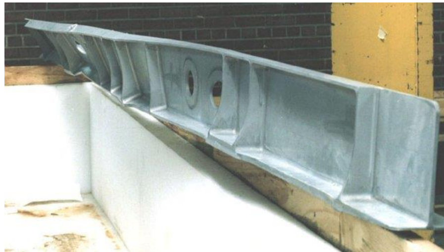
Extreme distortion caused by residual stresses
