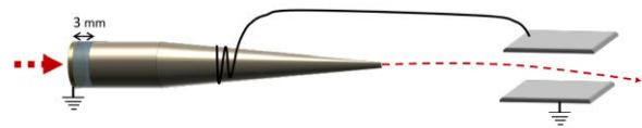
Figure 1. Electrode setup of conical-shaped borosilicate capillaries with deflection plates. The 3 mm insulator gap of about 10^{15} Ohm separates the grounded entrance from the floating electrodes.
