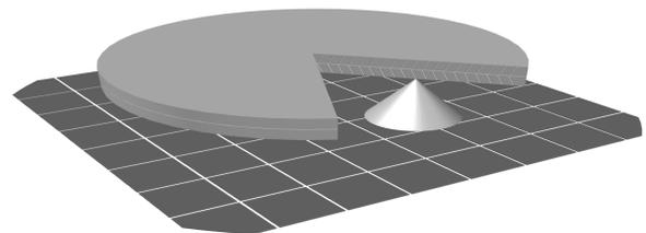
**Figure 2.** Gashed model of a MCP stack and a chessboard-like anode. The cone represents the trajectory of an electron cloud. Modified from [3].
