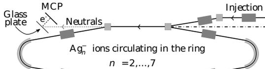
**Figure 1.** Schematic of the ion storage ring.
