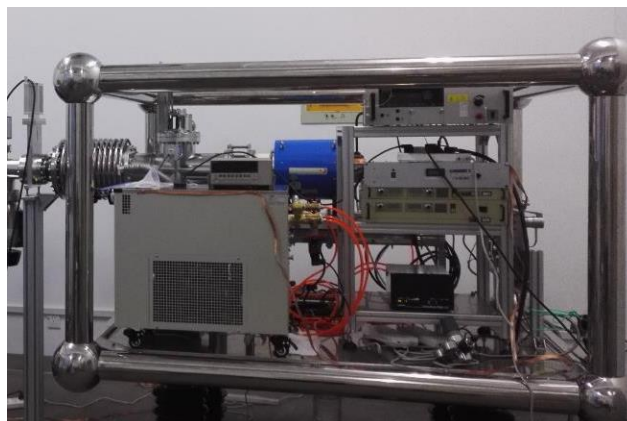
Figure 1. A photo of the 150 kV HCI research platform.
