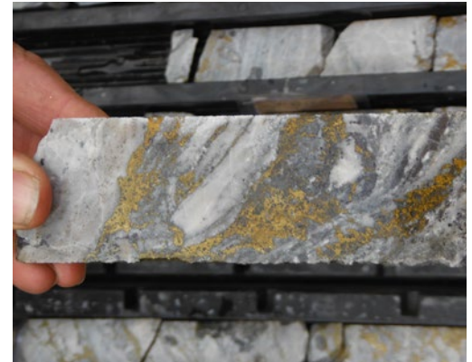
Chalcopyrite in drill core, Lala IOCG deposit, SW China. Lithium and REE are typically the first elements we think of as critical to achieving a carbon neutral future, but more mundane elements such as Cu, Ni and Co also feature high on national lists of critical materials.
