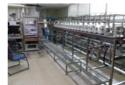
Water meter performance test corresponding to a given installation setup (15~50mm)
