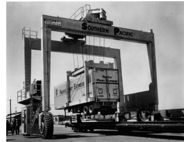
RTG in 1950s
