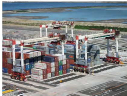
Rubber Tired Gantry Crane (RTG)
