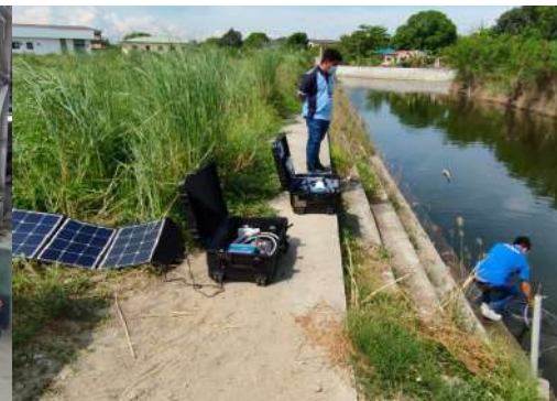
Testing of EWR box in a creek
