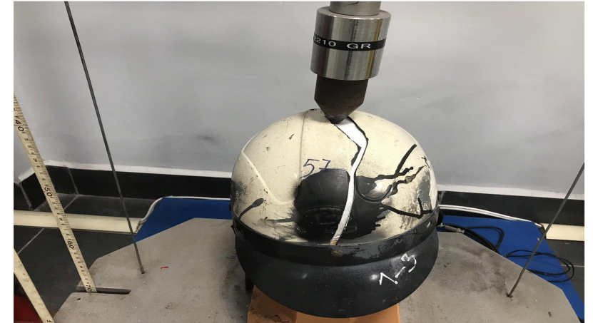
Half-face helmet splits in half during impact testing, despite passing all weight, size, and parts tests.
