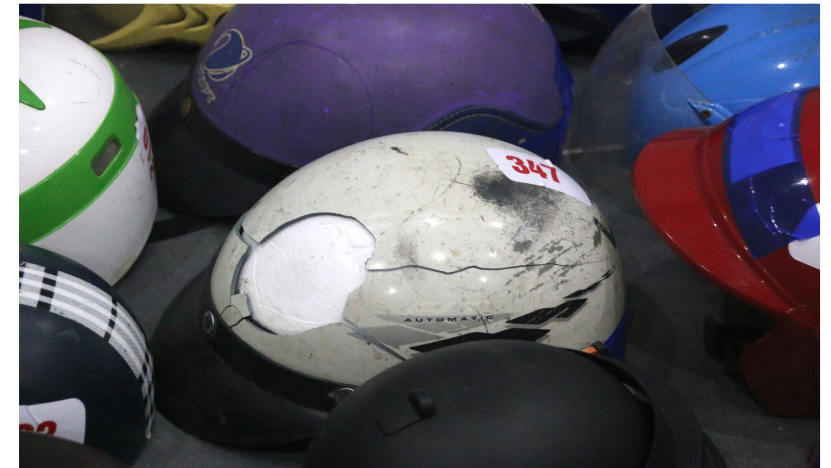
A helmet breaks during weight testing.
