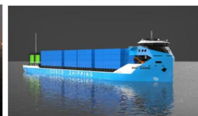
World's largest purely battery-powered 700TEU container ship – using swapable battery container
