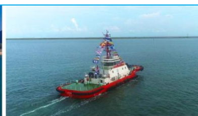
The first purely battery-powered tugboat in China Yungang Diantuo No.1
