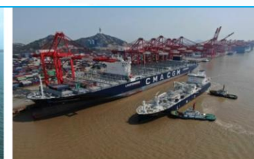
The first LNG bunkering SIMOP in China Shanghai Yangshan Port
