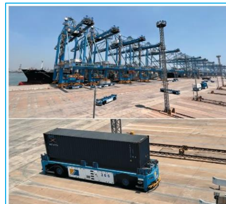
Equipment electrification. Electric automated guided vehicles are already operating in Qingdao Port (photo by Nestra).
