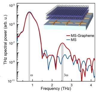
Fig.1. Measured spectrum of the THG at 2.5 THz generated inside two graphene sheets deposited on a metasurface (MS)-based bandstop filter (red line) and compared to the spectrum acquired with the MS alone (blue line). A highpass filter is used to reduce the driving field. Inset shows the sample schematic.
