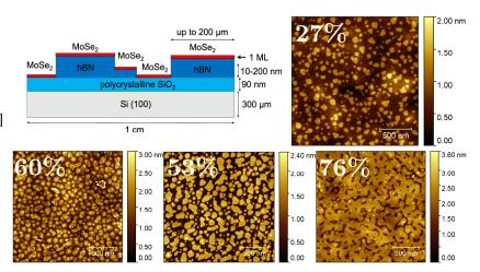
Fig. 1. Vertical sample cross–section [1] (top left) and AFM images of several MBE–grown MoSe<sub>2</sub> samples with different monolayer coverage factor.
