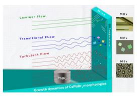
Fig.1. Impact of fluid flow (carrier gas) on selective and simultaneous growth morphologies.
