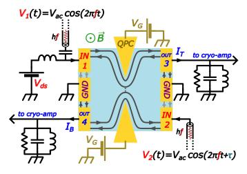
Fig. 1. QPC in a counter-propagating channels setup. Charge carriers excited by  $V_1$  and  $V_2$  (of time lag  $\tau$ ) are partitioned; transmitted and backscattered currents  $I_T$  and  $I_B$  are filtered by a 2.5  $\pm$  0.25 MHz LC circuit, ensuingly amplified by the cryogenic amplifiers. Signal is captured by a DAQ from with cross-correlations are computed. Additional details are found in [1].
