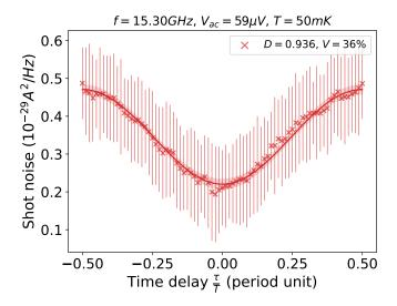
Fig. 2. HOM shot noise experiments shows that there is quantum coherence at  $\nu = 2/3$ . Visibility  $\approx 36\%$ . Measured data correspond to the  $\times$  symbols; the fit corresponds to the solid line.
