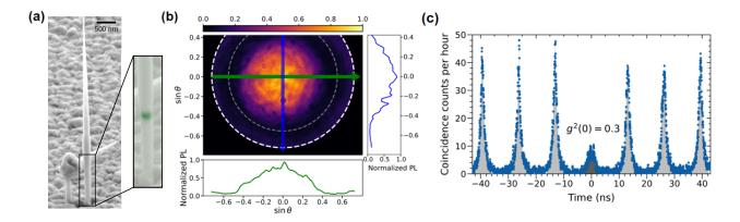
Fig. 1. (a) SEM image of a vertical and tapered ZnSe NW embedding a CdSe QD, with its position determined via a cathodoluminescence measurement. (b) Radiation pattern of the QD-NW emitter displayed in (a) through a microscope aperture of NA=0.72. (c) auto-correlation histogram of the one and same NW at 300K with a  $g^{(2)}(0)$  value of 0.3 at room-temperature.
