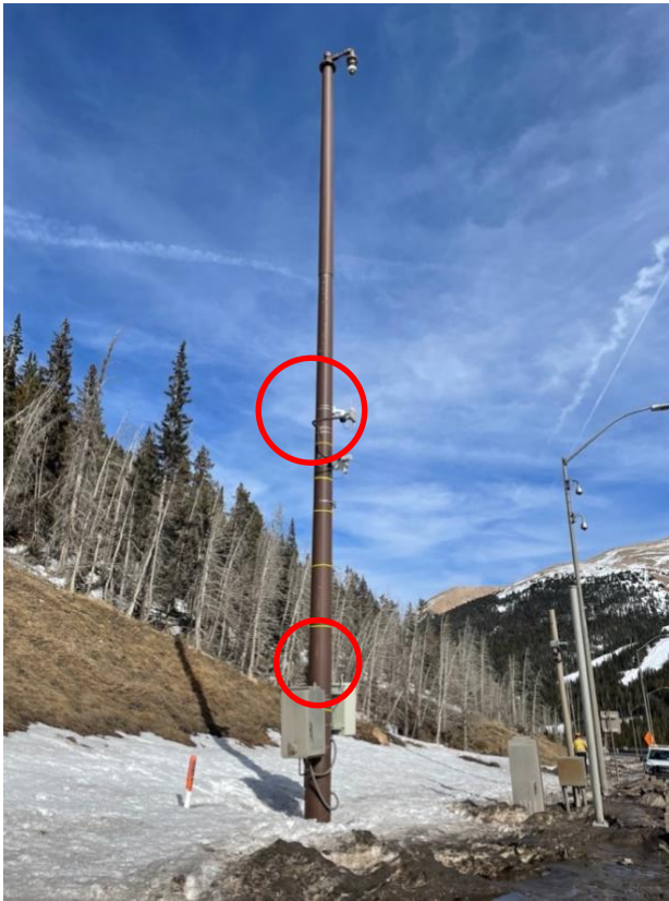
Figure 2: Installation of the AVYX Doppler radar at a camera pole of CDOT along I-70. The radar head and remote controllable PTZ camera were installed about halfway to the top at 4-5 m of elevation, the control cabinet just above the snow surface.
