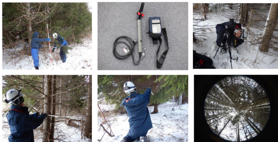
Figure 2: Tree observation in the shelterbelt: left, tree surveys; center, LAI using a PCA; right, LAI using a fisheye camera.
