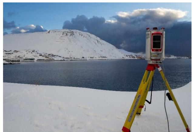
Figure 7: The TLS scanning the slopes above Honningsvåg in February 2021. Four ultrasonic sensors are located on the slopes visible in this photo.
