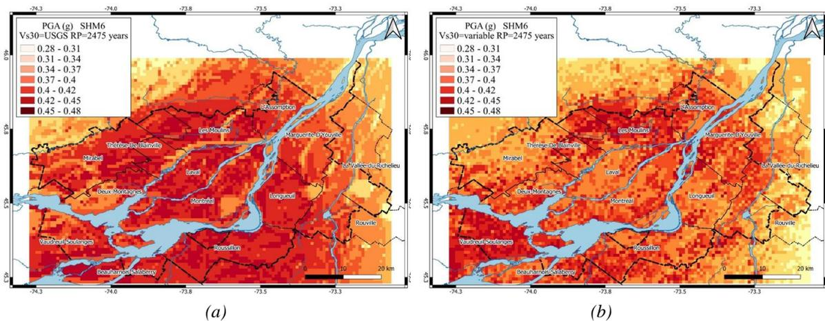
Figure 2. PGA (in g) calculated on a regular grid using SHM6 for the return period of 2475 years (probability of exceedance of 2% in 50 years) integrating the  $V_{s30}$  data in Figure 1 from (a) the USGS and (b) the detailed maps.
