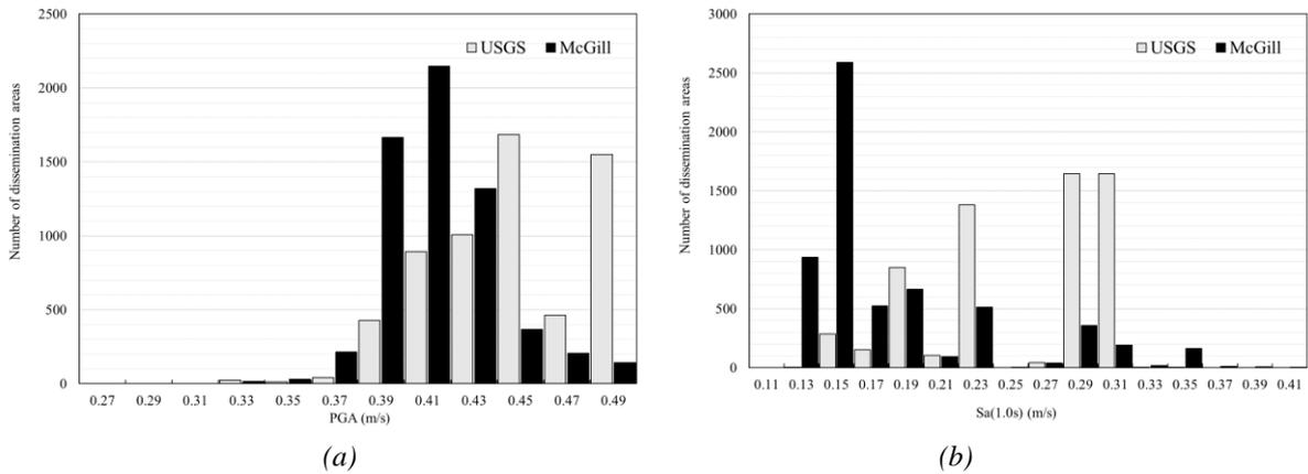
Figure 3. Distribution of calculated (a) PGA and (b)  $Sa(1.0s)$  by DAs using SHM6 for the return period of 2475 years (probability of exceedance of 2% in 50 years) and the  $V_{s30}$  models from USGS and McGill.
