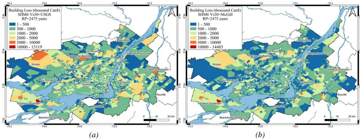
Figure 4. Residential building loss by DA calculated using SHM6 for a probability of exceedance of 2% in 50 years integrating the  $V_{s30}$  data in Figure 1 from (a) the USGS and (b) the detailed maps.
