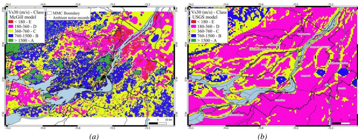
Figure 1. Site models in Greater Montreal in terms of  $V_{s30}$  (in m/s) grouped in site classes from (a) the detailed and (b) the USGS data.
