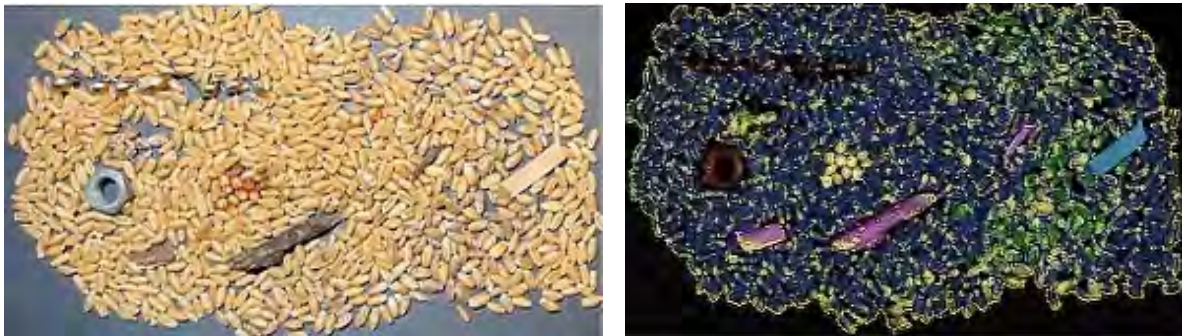
Figure 1 - Identification of impurities and moist/mouldy grains in wheat using hyperspectral imaging
