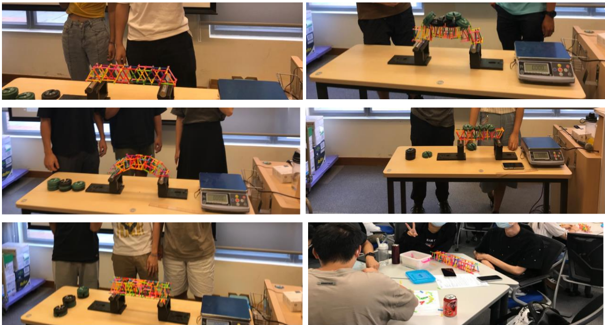
Figure 2: Assembly and loading test of plastic stick bridge challenge
