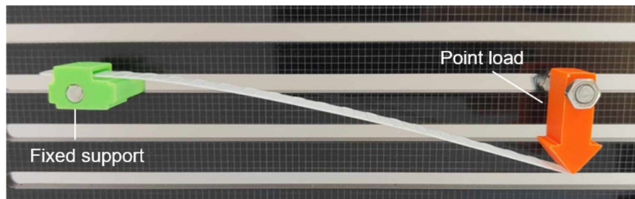
Figure 7: Deflection shape of a fixed cantilevered beam loaded at the free end using the PM.
