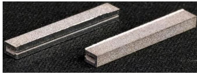
Figure 6: Fabricated samples of the leaky-wave antenna.
