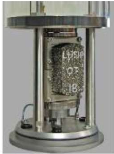
Texas Overlay Test
