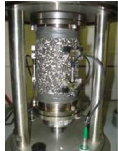
Direct Tension Cyclic Fatigue, S-VECD
