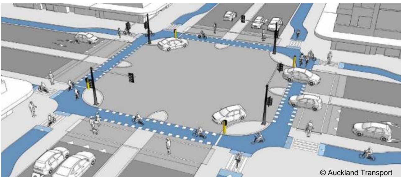
Figure 8: Suggested arterial road treatment
