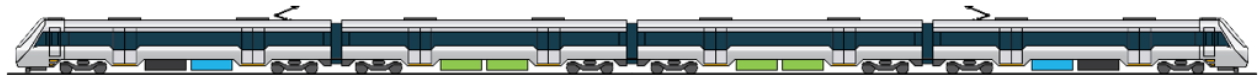
Underfloor layout proposed in LNIRIM DBC: 1.6kV DC equipment in blue, Batteries in green, CI engine/genset in black
