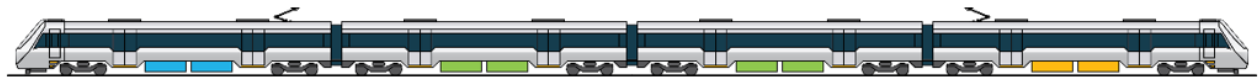
INTEGRATOR MODE: Due to advancing battery technology, this rolling stock underfloor layout, will become viable regarding range resilience, at the time of procurement and/or future fleet upgrade: 1.6kV DC equipment in blue, 25kV AC equipment in gold, Batteries in green
