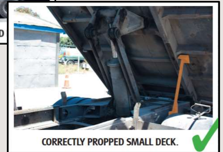
Deck Props Fitted To Big and Small Truck Decks (A Certified Safe Initiative)
