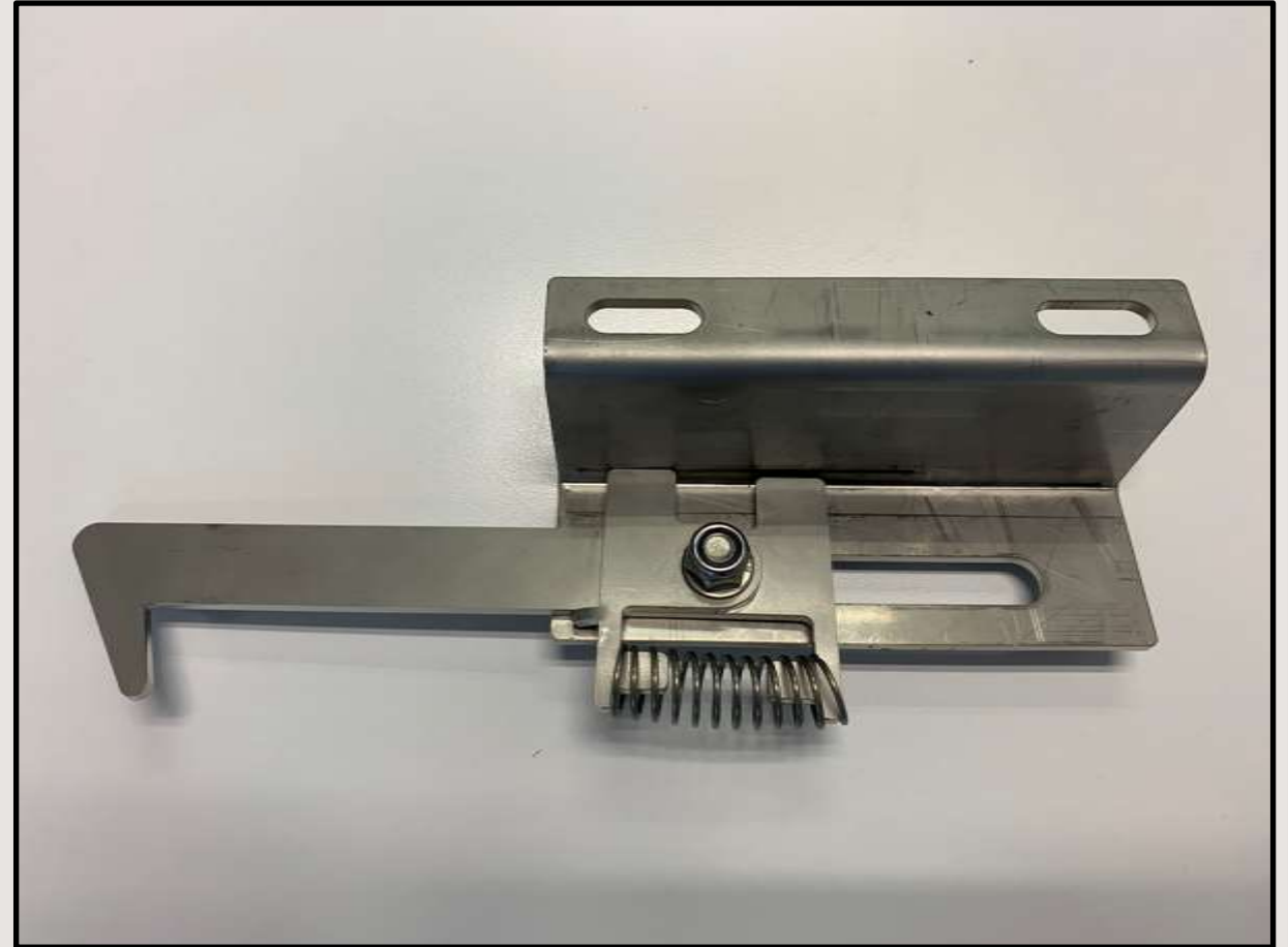
Secondary lock to truck cabinet doors – designed and implemented through the Fulton Hogan Certified Safe programme in 2021.
