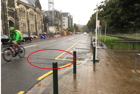
Figure 3: tubes miss all right turning cyclists (Christchurch)
