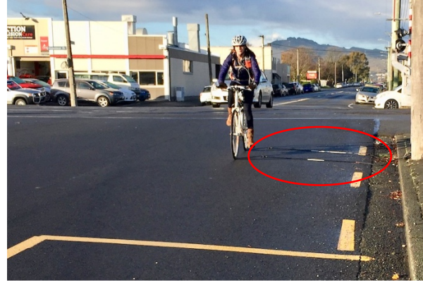
Figure 4: tubes miss most riders due to parking lane alignment (Christchurch)
