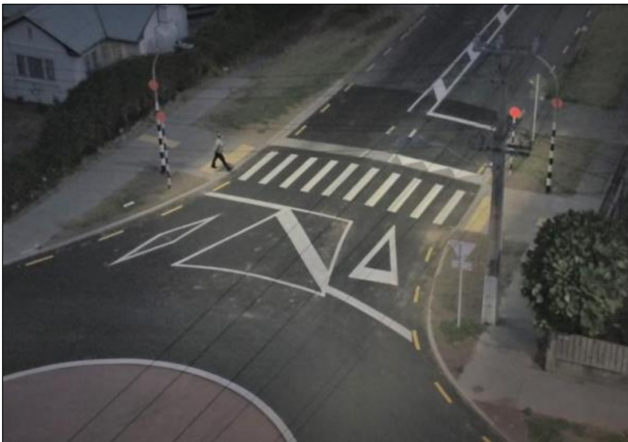
FIGURE 7: NEW PEDESTRIAN CROSSING WITH STREET LIGHTING
