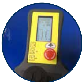
Joystick control of hydraulic functions and rotor speed
