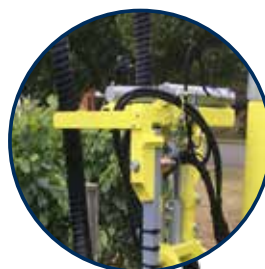
Breakaway system to protect the frame
