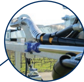
Double beam for improved mast strength. Rollers ensure heads are easily adjustable for different row widths. Optional hydraulic row width adjustment kit is now available
