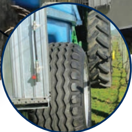
Wider profile tyres ensure less ground compaction and improved stability
