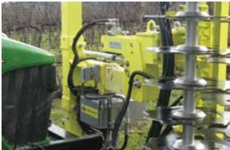
Equipped with a robust frame with two 16cc hydraulic motors.
