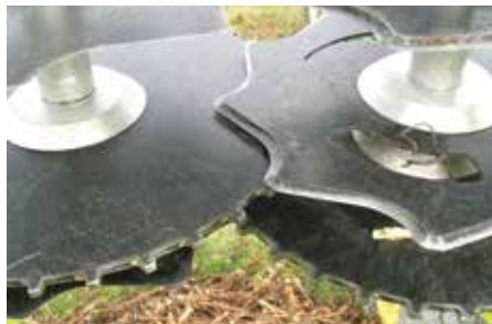
Blade and notched discs for efficient clean cuts and trellis post protection.
