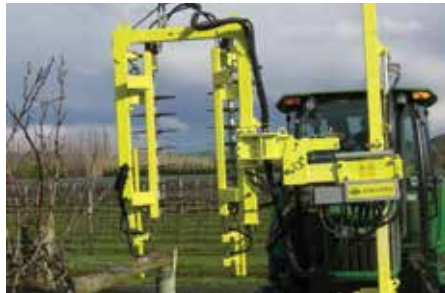
Three hydraulic functions, up/down, in/ out and cross slope.
