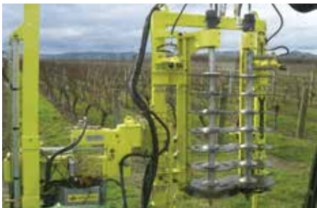
Modular cutting height up to 825mm. 80 or 110mm blade spacings.
