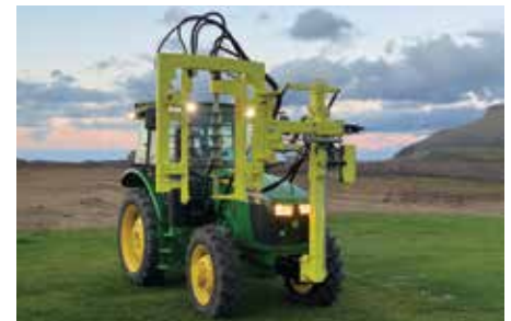
Manual folding system (AVR model) by articulation in front of the tractor, for safe road transport.
