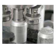
Pre-threaded caps: suitable for the application of the pre-treated caps on glass or plastic bottles. Application is done by picking the cap from the feeding mechanism, with the capping head chuck, placing and screwing it on the bottle with desired torque, called pick and place method.
