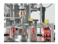
Twist-off caps: suitable for the application of the twist-off lug caps on glass bottles. Caps are picked by the bottles and tightened with the capping head to the desired torque. Capping is done in steam environment, steaming the cap and bottle neck, steam in the bottle neck which will positively affect the vacuum inside the bottle
