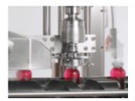
Crown caps: suitable for the application of the crown caps on glass or aluminum bottles. The cap is applied by deforming it with the help of closing cone, so the cap will clamp the bottle neck. Addition applications for bidule insertions is possible before crown capping.
