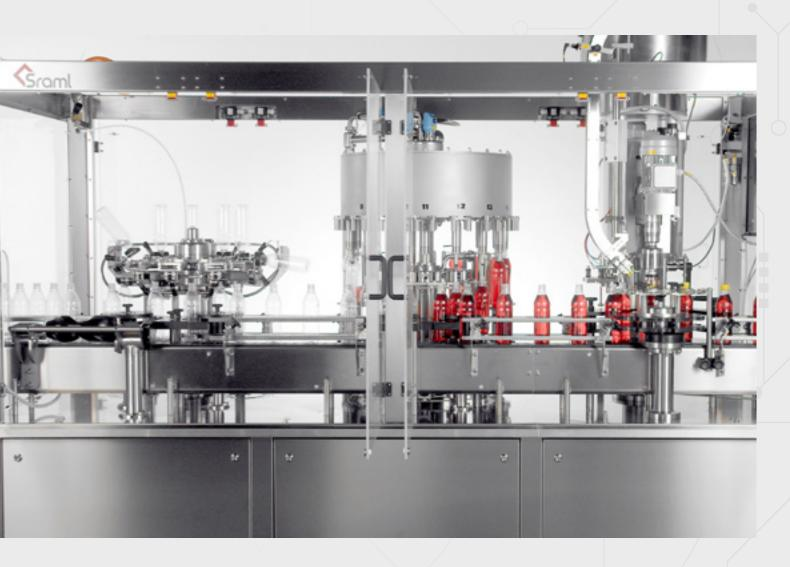
Designed to execute different tasks in the bottling process while forming part of the same block, a monoblock system has several advantages compared to individual, stand-alone machines connected by conveyor belts since it requires less space and personnel, optimises energy consumption, and enables perfect synchronization between units.
