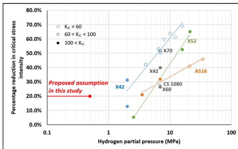
Figure 1: Logarithmic plot of toughness reduction (%reduction in  $K_{IC}$ ) created from data from the Sandia technical databases for hydrogen compatibility of materials (San Marchi & Somerday, 2012) (Ronevich & San Marchi, 2021)
