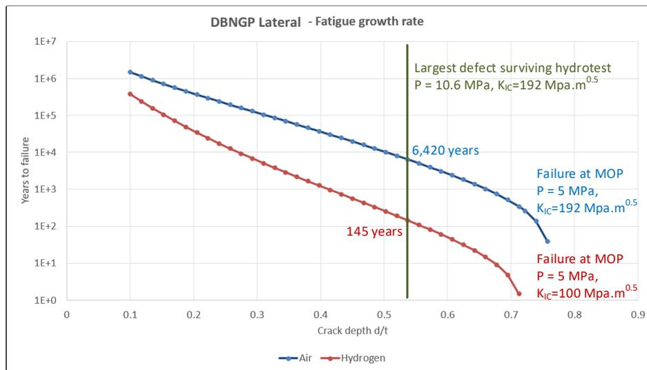
**Figure 6: Fatigue life for infinite length crack of depth  $d$  at MOP of 5 MPa**
