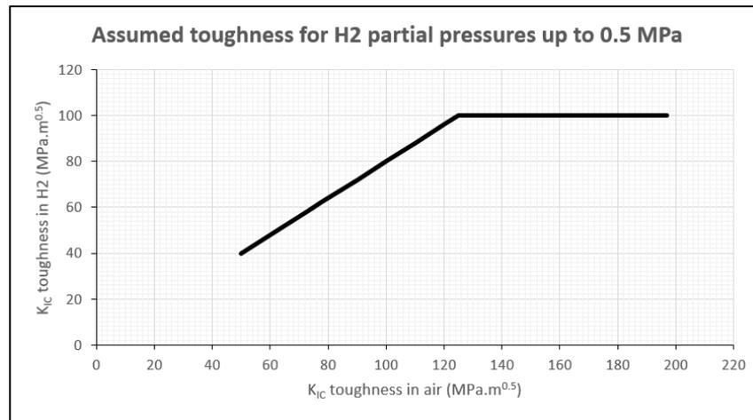
Figure 2: Conservative assumed toughness ( $K_{IC}$ ) reduction for hydrogen partial pressures up to 0.5MPa
