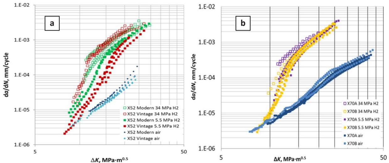
Figure 3: Fatigue crack growth rate of (a) X52 and (b) X70 steels at pressures of 34 MPa and 5.5 MPa (Slifka, et al., 2018)
