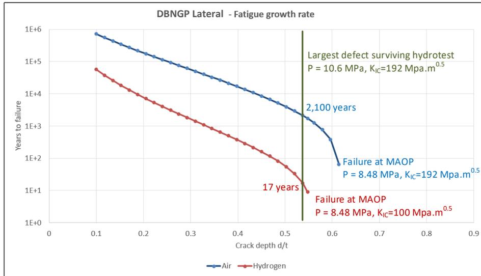
**Figure 5: Fatigue life for infinite length crack of depth  $d$  in DBNGP Lateral at MAOP**
