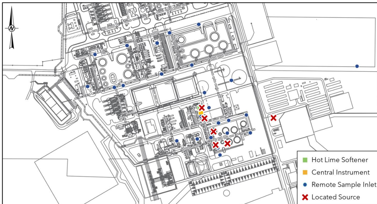
Figure 5. Configuration of the continuous monitoring system and site layout of the SAGD facility, including the location of important emission sources identified through the analysis.
