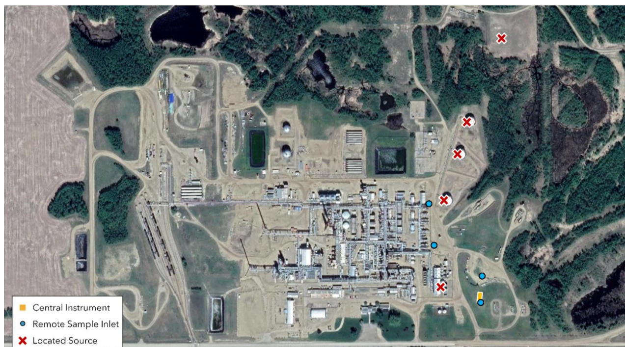
Figure 3. The layout of the midstream oil and gas facility with the set-up of the continuous monitoring system and the located onsite and offsite emission sources.
