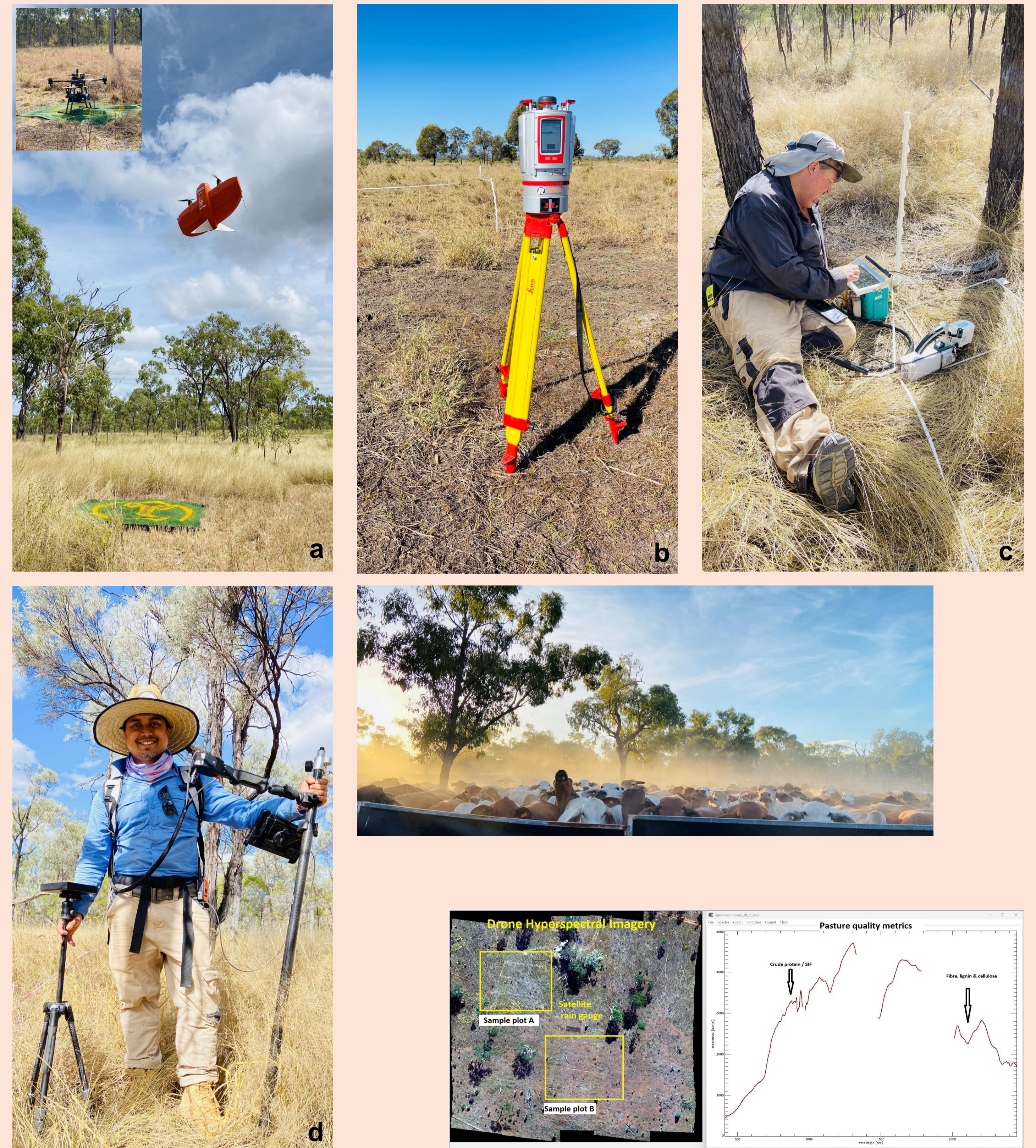
Figure 2: Field measurements of pasture quality and quantity by Dr Jason Barnetson (DES researcher) and Dr Hemant Raj Pandeya using a) uncrewed aerial vehicles (UAVs) b) terrestrial 3D laser scanner c) portable LI-COR 6800 instrument d) RS-8800 field spectroradiometer.
