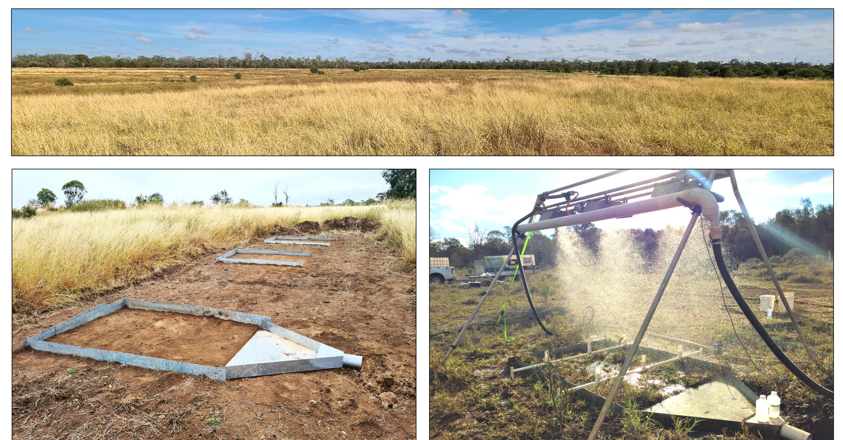
Figure 2. Fitzroy Basin grazed hillslope (top). Rainfall simulation plot 1.4m by 2m long prepared as a scald plot (left). Rainfall simulation in action over a vegetated plot (right).
