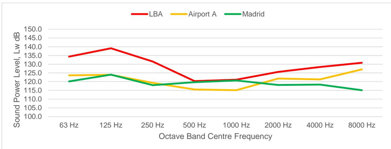
Figure 4: A319 - Octave band centre frequency sound power levels,  $L_w$  (average differences, dB)
