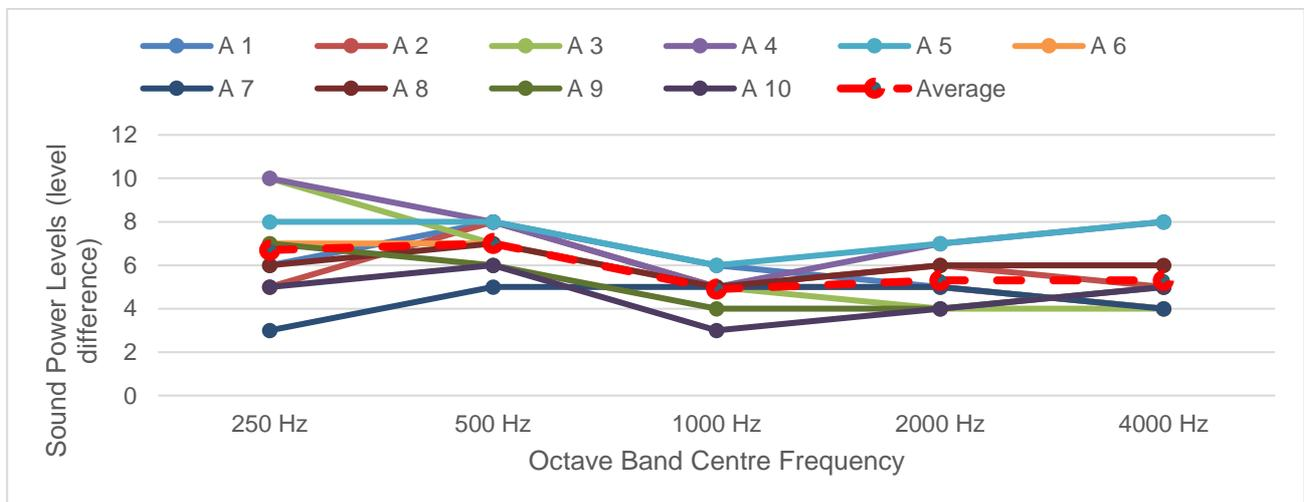
Figure 2: Airport A A319 - Sound power level,  $L_w$  (level differences, dB)
