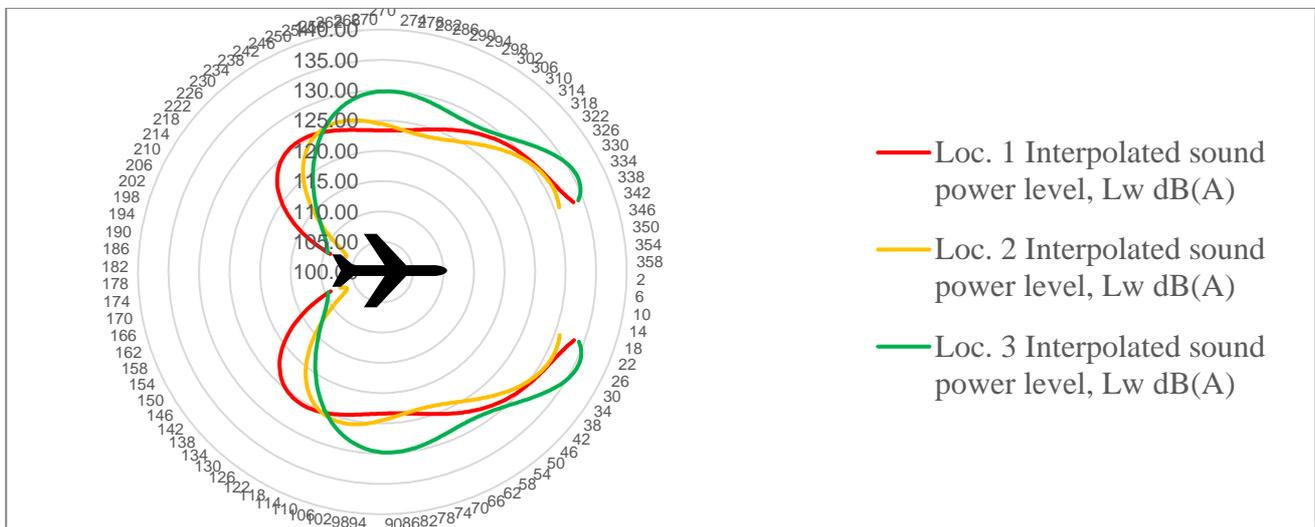
Figure 3: LBA A319 - Sound power level,  $L_w$  (directivity differences, dB)
