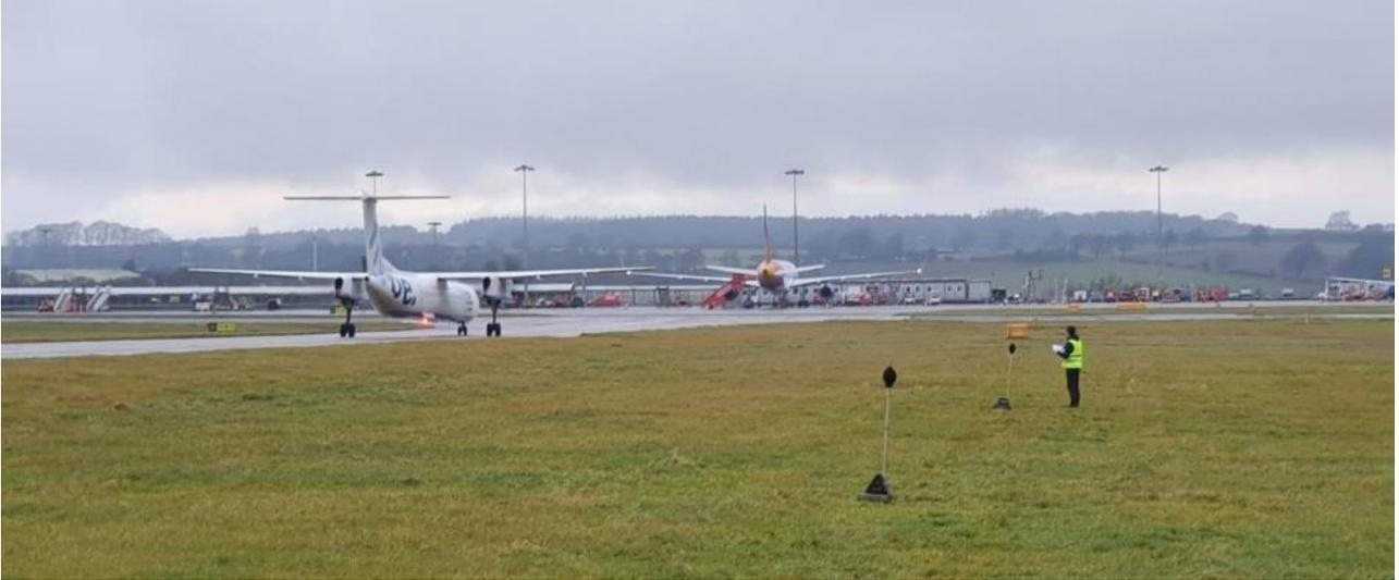
Figure 1: Photograph: LBA - taxiing aircraft in noise measurement array
